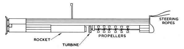
Figure 3. The Berdan Rocket Torpedo, c1885
