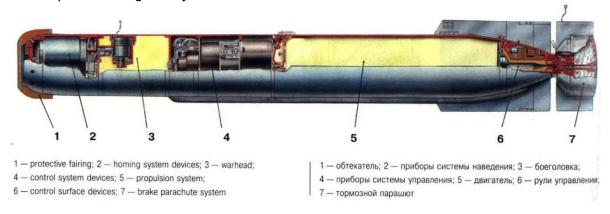
Figure 13. Russian APR-2E rocket torpedo
