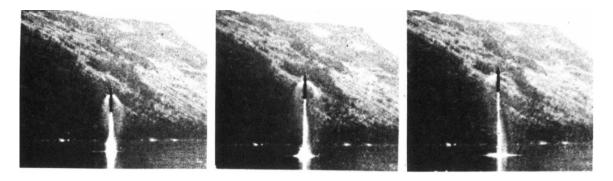
Figure 8 Sequence of still shots showing torpedo breaking surface
